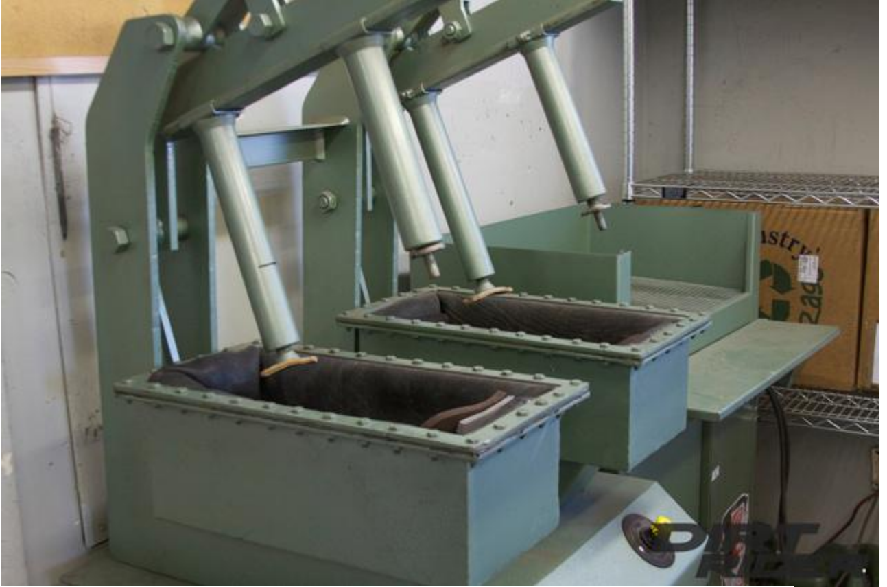
This is the special, all-around press machine that makes replacing the factory Alpinestars molded soles possible.
