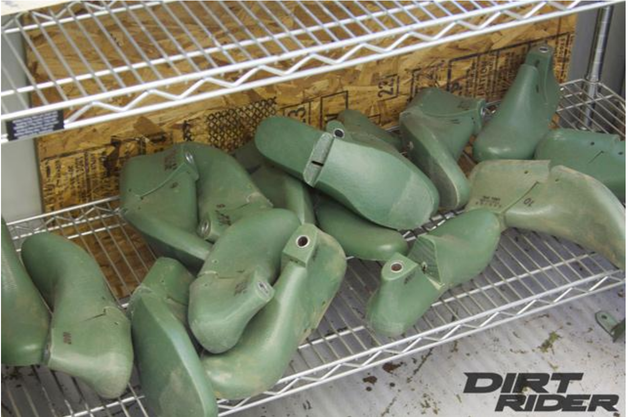
To insure that the boots don't collapse in the press, each needs a plastic foot mold installed.
